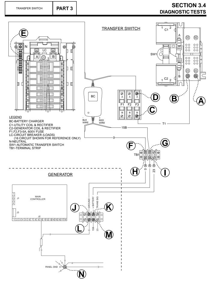
Figure 11. Test 40, 41, and 42 "Pre-Wire Load Center" Test Points.
